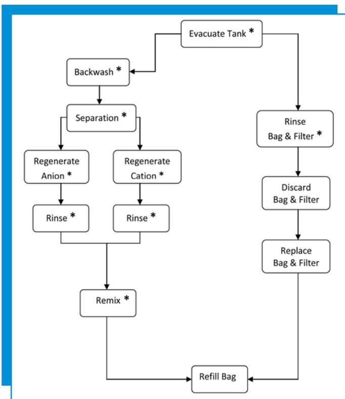
Fig #4b Bag regeneration process diagram
