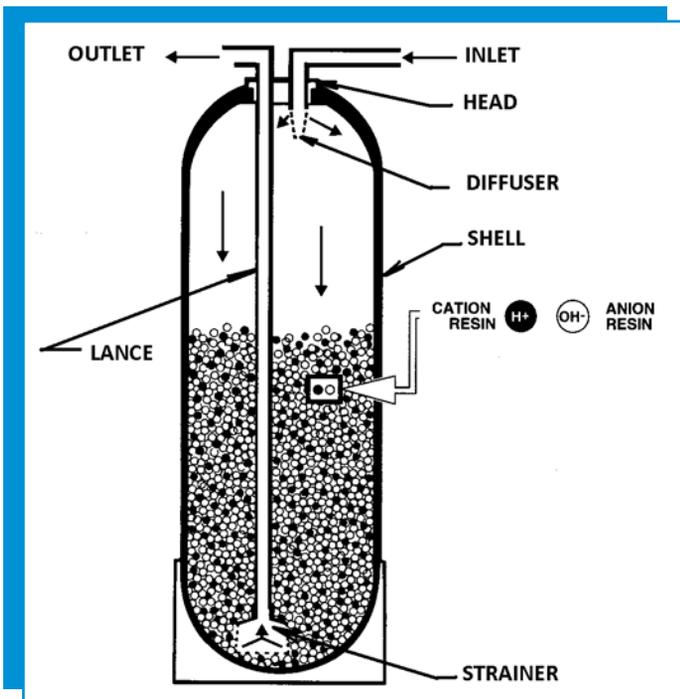
Fig #2b: Cross section of fiberglass resin tank
