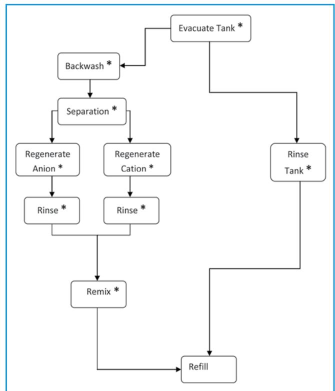
Fig #4a Tank regeneration process diagram
