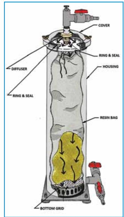
Fig #3c: Cross section of Ebbco style bag housing
